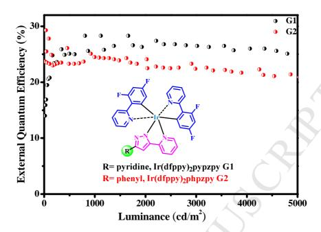
Efficient sky-blue OLEDs based on two irdium(III) complexes show a maximum luminance of 38 200 cd/m<sup>2</sup>, a maximum current efficiency of 58.74 cd/A, a maximum power efficiency of 49.85 lm/W and a maximum external quantum efficiency of 29.30%, respectively, with low efficiency roll-off.
