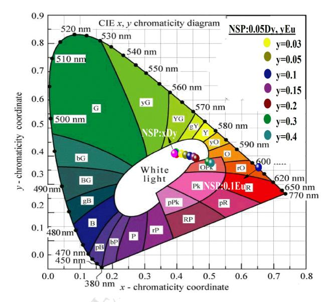
Tunable white emissions were achieved in Dy<sup>3+</sup> and Eu<sup>3+</sup> co-doped Na<sub>3</sub>Sc<sub>2</sub>(PO<sub>4</sub>)<sub>3</sub> phosphors for near-UV LED-based warm white LEDs.
