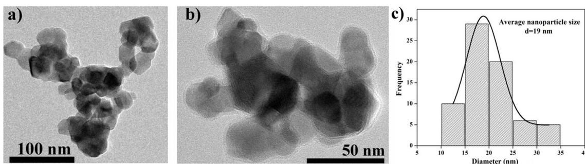
**Fig. 1.** a) and b) Typical TEM images for un-doped YOF nanoparticles at two different magnifications; c) size distribution histogram of YOF nanocrystals.
