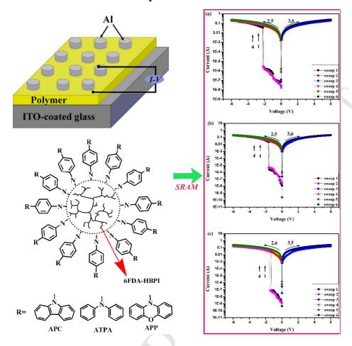
Three functional hyperbranched polyimide (HBPI) terminated by APC, ATPA and APP were synthesized and employed to act as the building block of the memory device, which exhibited tunable performances along with the change of the terminal group.
