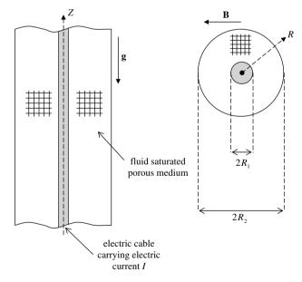
Fig. 1. Drawing of the vertical annulus.
