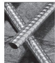
Fig. 1. Experimental setup and the enhanced tubes. (a) Schematic of the experimental setup, (b) fins on Turbo-CAB tubes, (c) Turbo-CAB-19 fpi, and (d) Korodense.
