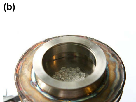
Fig. 1. (a) The basic 3T cycle of AHP in the Clapeyron diagram. (b) The measuring cell with loose grains on the metal support exposed to temperature jump/drop.
