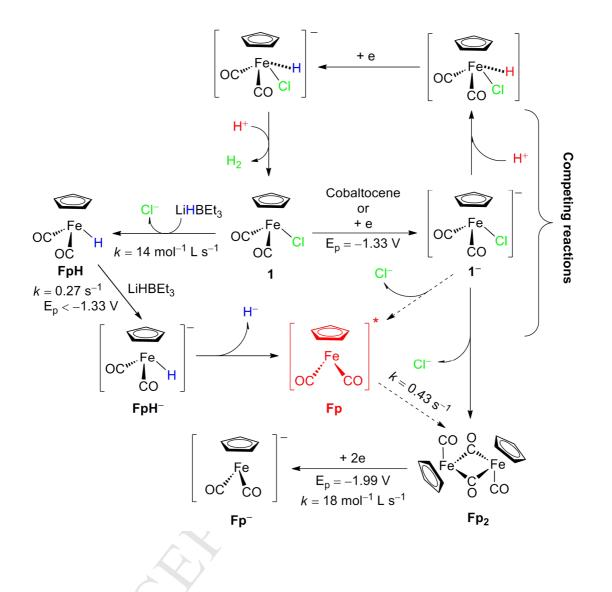
By using cyclic voltammetry and stop-flow infrared spectroscopic technique combining with chemical reduction, the electron transfer process of half-sandwich iron(II) complex **1** and coupled chemical reaction were well established and kinetic parameters for related reactions were derived.
