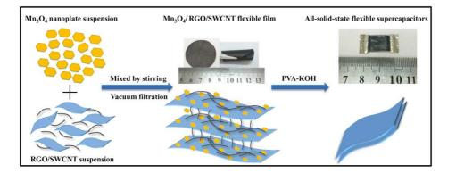
All-solid-state  $Mn_3O_4/RGO/SWCNT-50$  flexible symmetrical supercapacitor is developed by using PVA–KOH gel electrolyte, it shows high energy density and good flexibility property.
