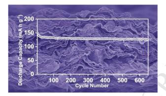
The binder-free films of hollow  $Na_2Ti_3O_7$  spheres and reduced graphene oxide showed excellent rate performance and good durability as flexible anodes for sodium ion batteries.
