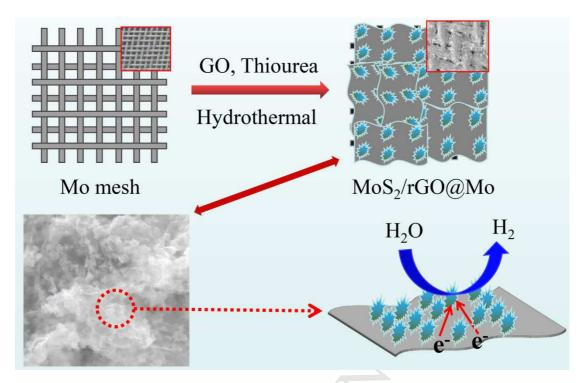
3D MoS<sub>2</sub>-rGO@Mo catalyst was fabricated by a sample one-pot hydrothermal process, which exhibits excellent HER performance in alkaline solution.
