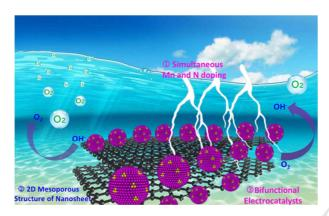
Mn doping of cobalt oxynitride ( $Co_{1-x}Mn_xON$ ) coupled with nitrogen-doped reduced graphene oxide (N-rGO) nanosheets hybrid is created as a highly efficient and bifunctional electrocatalysts toward ORR and OER. The CoMnON/N-rGO hybrid catalyst manifests excellent catalytic performace, durability, and good methanol-tolerance ability.
