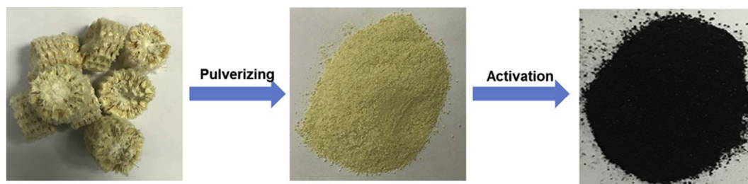
Scheme 1. Schematic procedure for the preparation of biochar from corncob.
