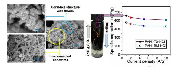
The as-prepared polyaniline exhibits a bimodal morphology composed of a coral-like structure and a nanowire structure. A large specific capacitance of 689 F/g at 1A/g and retention of 613 F/g at 10 A/g is obtained for net polyaniline.
