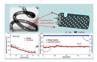
Unique spiral morphology, high defect degree and dominated pyrrolic N endowed PN-CFs with superior cycling stability and rate capability.
