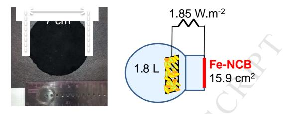
Iron-Nicarbazin derived platinum group metal-free electrocatalyst was incorporated into a scalable-size air-breathing cathodes and tested in microbial fuel cells. Maximum power density of 1.85 W  $\text{m}^{-2}$  was achieved initially and then decreased to 1.25 W  $\text{m}^{-2}$  after 22 days operations.
