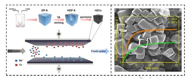
Hollow ZIFs-derived porous carbons (HZCs) was prepared via chemistry etching method and subsequent pyrolysis, then utilized as CDI electrodes. The as-prepared electrode exhibits excellent capacitive deionization performance and great stability.
