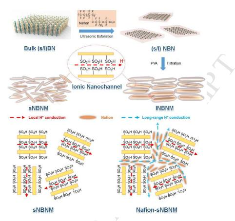
Stable and selective membranes with novel ionic nanochannels based on functionalized two-dimensional boron nitride nanocomposites (NBN) are successfully fabricated
