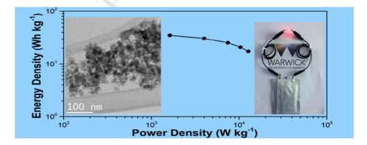
Nanoporous nickel-copper sulfide on carbon cloth is prepared as positive electrode materials for high-performance supercapacitors.
