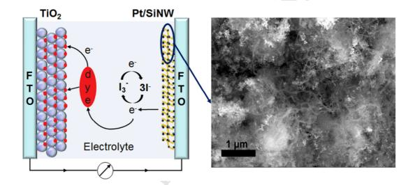
Pt nanoparticle/Si nanowire composites are employed as the counter electrode in dye-sensitized solar cells. Si nanowires prevent metal nanoparticles from agglomeration. The density functional theory calculation shows that the adsorption energy of I atom on the Pt/Si interface is -0.8 eV, which is the optimal adsorption energy for triiodide reduction. The power conversion efficiency of device based on the Pt/SiNW electrode is 3.8% higher than that of the device based on Pt.
