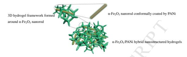
PANi coating is in situ polymerized on the  $\alpha$ -Fe<sub>2</sub>O<sub>3</sub> surfaces and well interconnected hierarchical porous PANi framework form simultaneously.
