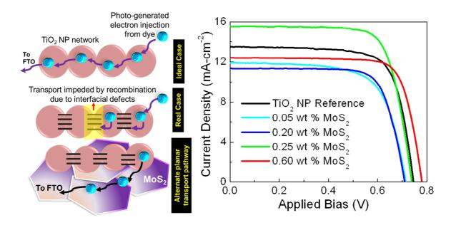
2D Layered MoS<sub>2</sub> in TiO<sub>2</sub> facilitates charge transport and improves DSSC performance
