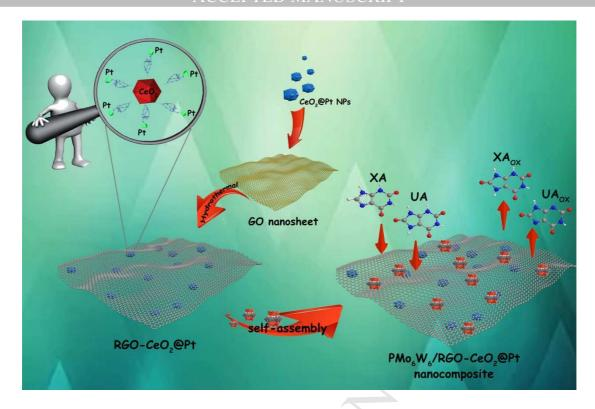
A new nanocomposite was fabricated by combining 12-heteropolyacids ( $PMo_6W_6$ ) and  $CeO_2$  decorated by Pt nanoparticles and RGO. Enhanced electrocatalytic activity and sensing performance were achieved due to the synergistic effect of components in nanocomposite. The proposed  $PMo_6W_6/RGO-CeO_2@Pt$  is promising material for simultaneous or individual detection of xanthine and uric acid in practical application.
