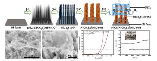
An active and stable bifunctional NiCo/NiCo<sub>2</sub>S<sub>4</sub>@NiCo/Ni Foam electrocatalyst based on the unique mushroom-like structure and the beneficial effect of composite.
