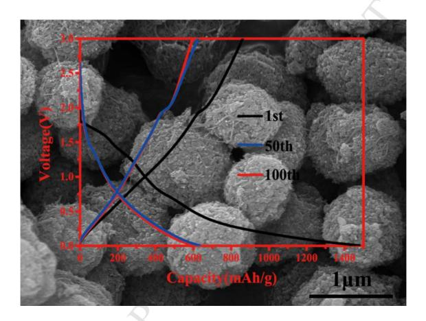
The C/NiO hollow microspheres successfully obtained by using yeasts bio-template and glucose as carbon source have demonstrated higher discharge capacity and better cycle performance as an anode material in Li-ion battery.
