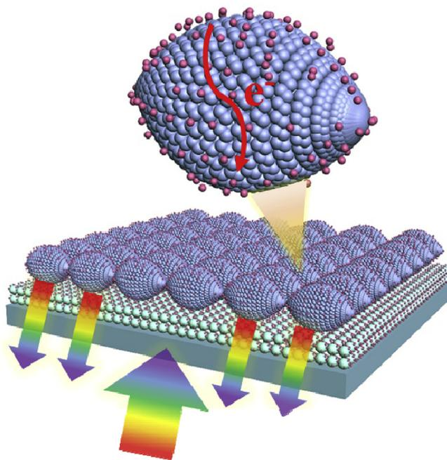
**Scheme 1.** A schematic diagram of the bi-layer photoanode with MCs scattering layer on top of the nanocrystalline underlayer.
