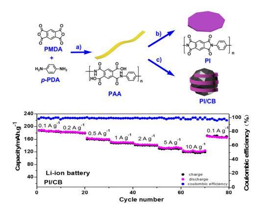
**Composites as High Performance Lithium Ion Battery Cathodes**
