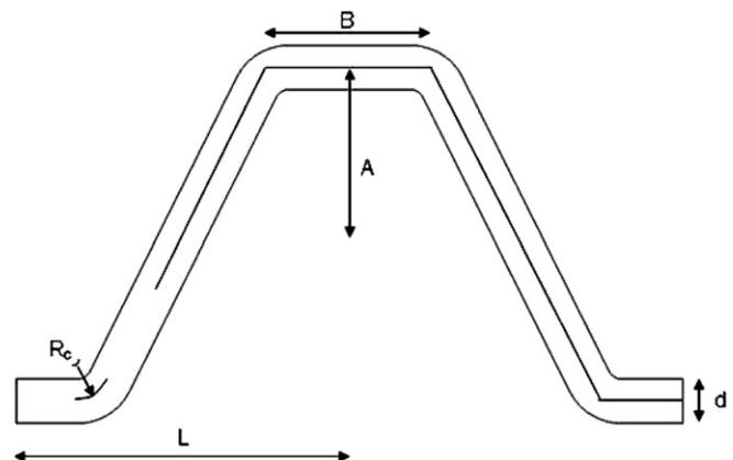
Fig. 1. The dimensions of the trapezoidal unit.  $L$  is the unit half length,  $d$  is the length of the side of the triangle,  $R_c$  is the radius of curvature,  $A$  is the half height of the trapezoid and  $B$  is the length of the top run.
