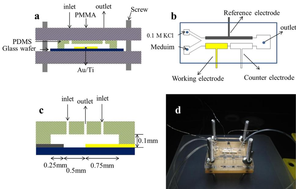
**Fig. 1.** Scheme of the microfluidic channel device. (a) Front view. (b) Top view. (c) Side view. (d) A photograph of the assembled device.
