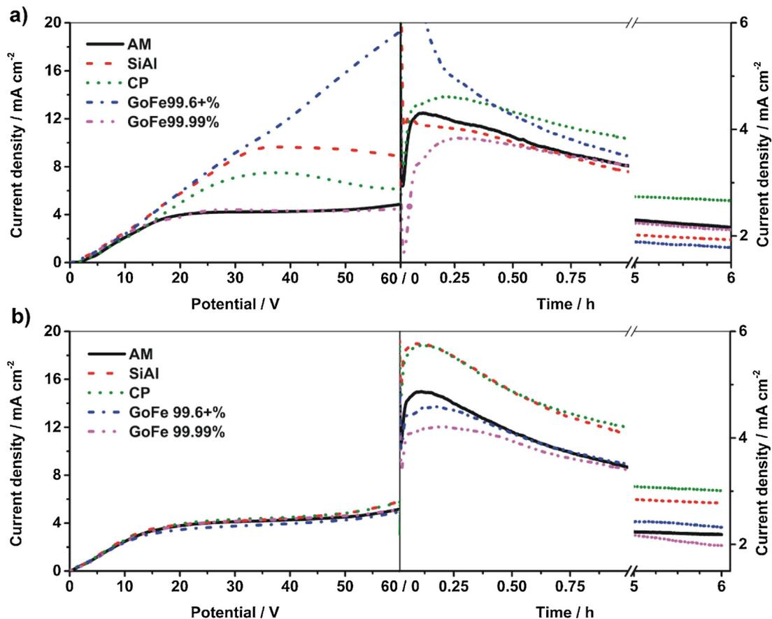
**Fig. 1.** Polarization plots (left) and current transients (right) recorded for the anodization of different Ti substrates for the 1<sup>st</sup> anodization (a) and for the 2<sup>nd</sup> anodization (b). The curve for the 1<sup>st</sup> anodization shows the initial 6 hours of the total time of 14 hours.
