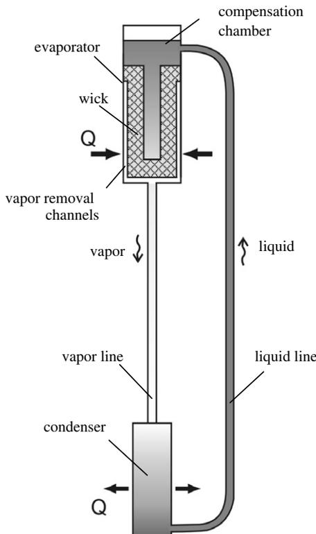
Fig. 1. Scheme of a loop heat pipe.
