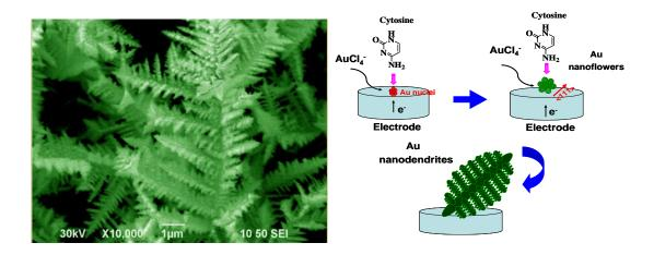
In this work, Au hierarchical dendrites (HDs) were prepared by one-step electrodeposition with the assistance of cytosine. This approach is simple, fast, feasible, controllable and cost-effective, without any template or surfactant. The as-prepared Au nanocrystals were applied for SERS amplification detection of Pb<sup>2+</sup> with high sensitivity.
