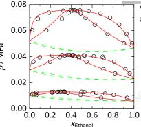
Vapor-liquid equilibria on three isotherms for a binary mixture of ethanol + benzene
