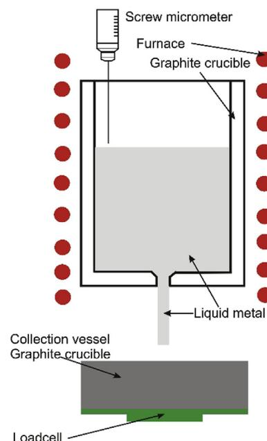
Fig. 1. Equipment for simultaneous measurement of density, surface tension and viscosity.
