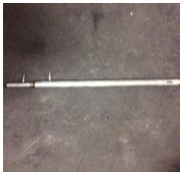
Fig. 1. Diagram of experiment system: (a) Schematic diagram of the drop tube furnace system; (b) Photo of water-cooled ash deposition tube.
