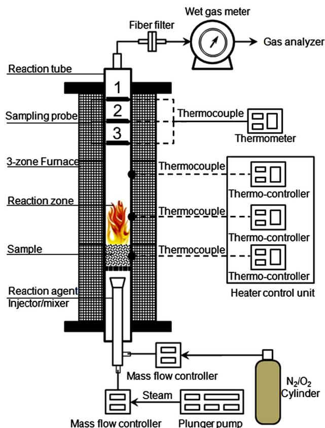
Fig. 1. Schematic diagram of pressurized fixed bed pyrolysis/gasification reactor.
