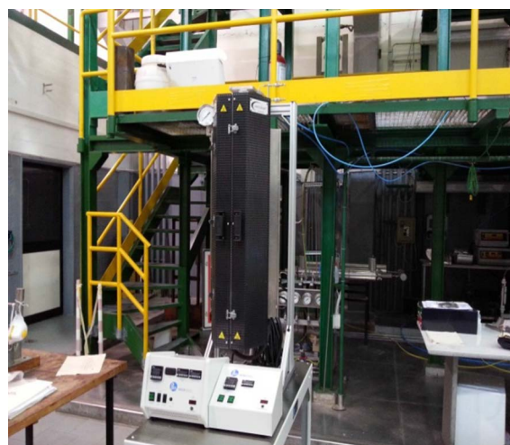
Fig. 2. Bench scale SCWG reactor.
