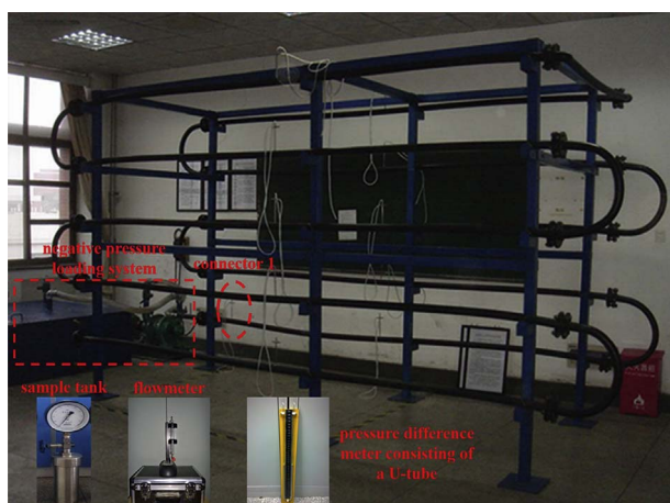
Fig. 2. Physical image of the negative pressure pipeline equipment.
