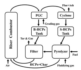
Fig. 1. Principle of the DLRS reaction system (B-HCPs: Big Heat Carrier Particles; S-HCPs: Small Heat Carrier Particles; PGC: Particles Grading Cyclone).
