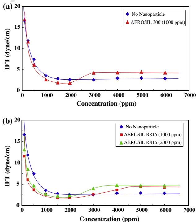
**Fig. 2.** Oil/water interfacial tensions for aqueous nanoparticle-augmented surfactant solutions of different surfactant concentrations at constant nanoparticle concentrations. (a) AEROSIL 300, and (b) AEROSIL R816.
