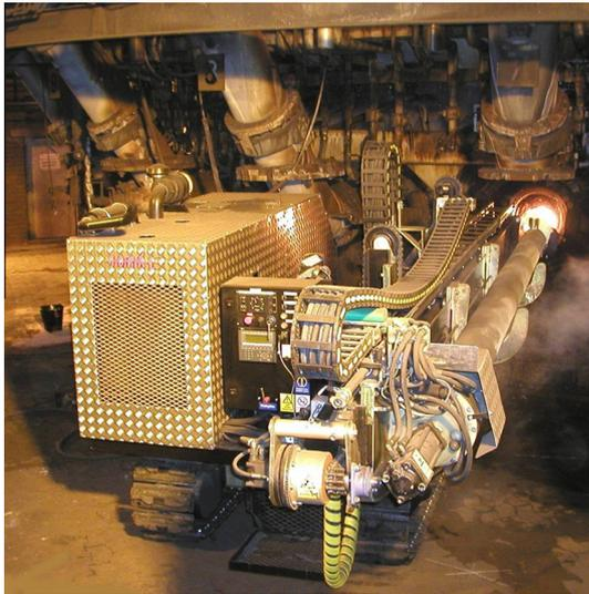
**Fig. 1.** Mobile tuyere drilling probe.
