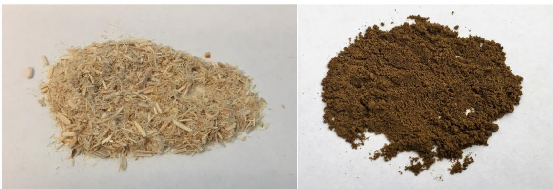
Fig. 1. Picture of pine sawdust particles (left) and microalgae particles (right) at 10% wet basis moisture content.
