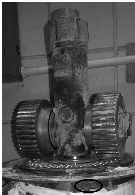
Fig. 1. Pilot scale flat ring roller pellet mill with shielding removed showing rollers and location of thermocouples on die (circled).
