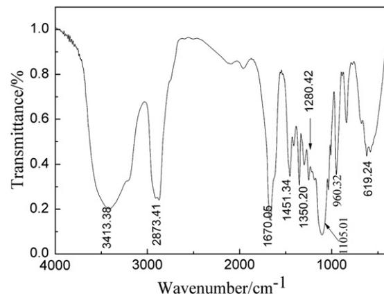
Fig. 3. FTIR spectrogram of long side-chain polycarboxylate dispersant ( $m = 14$ ).
