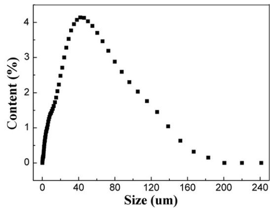
Fig. 2. Particle size distribution of Shenfu coal sample.
