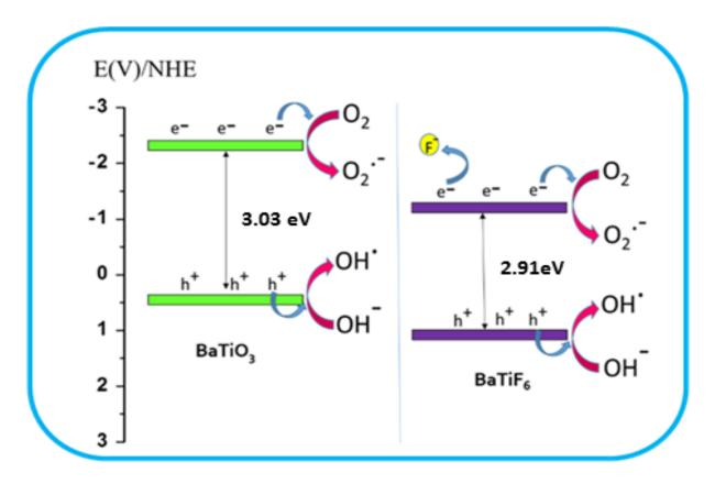
Suitable band edge positions, higher surface area and porosity, higher surface acidity, higher absorption co-efficient and efficient charge trapping makes  $BaTiF_6$  a better photocatalyst under both UV/solar light irradiation.
