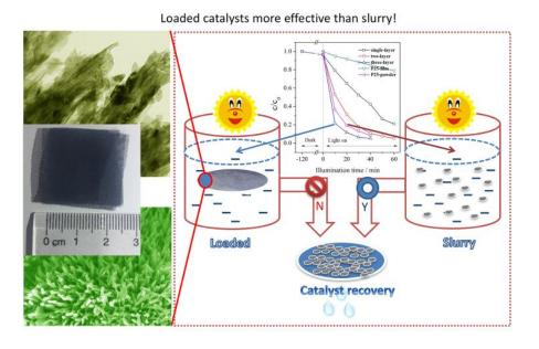
A novel low temperature approach was developed to synthesize few-layer titanate nanobelts on metallic Ti mesh. After a subsequent hot water treatment, titania nanorods were achieved. The loaded titania exhibited a photocatalytic activity superior to that in a P25 slurry system.
