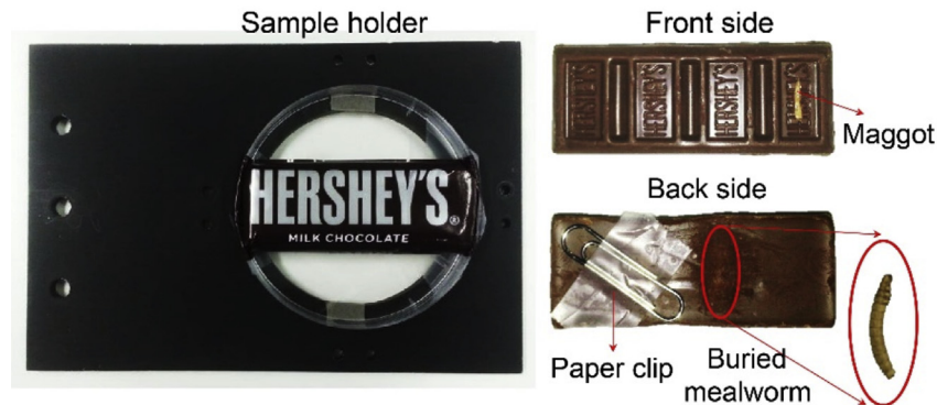
Fig. 1. Left: Wrapped chocolate bar with the foreign bodies on the circular sample holder. Right: Foreign bodies embedded in the chocolate bar, where the dried maggot was attached to its front side, the paper clip was on its back side, and the mealworm was buried inside it. The image of the chocolate bar is reproduced with the permission of the Hershey Company.
