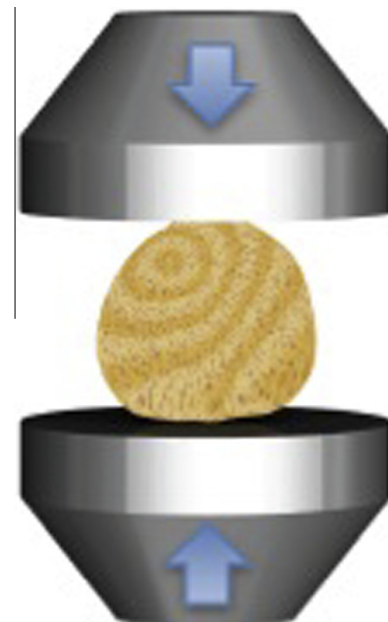
Fig. 2. Kernel compression along A axis, experimental setup.
