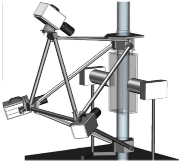
Fig. 1. Schematic of the 3D-PTV experimental setup for particle-laden pipe flow.
