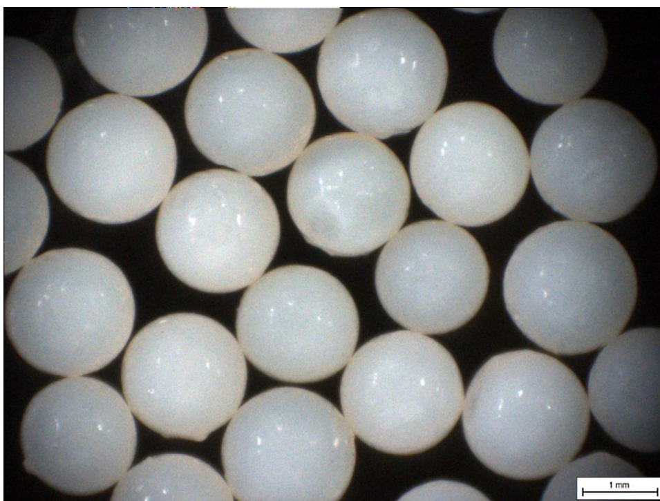
Fig. 1. Optical photograph of \gamma -AlOOH/PVA composite granules with 35 wt% PVA.
